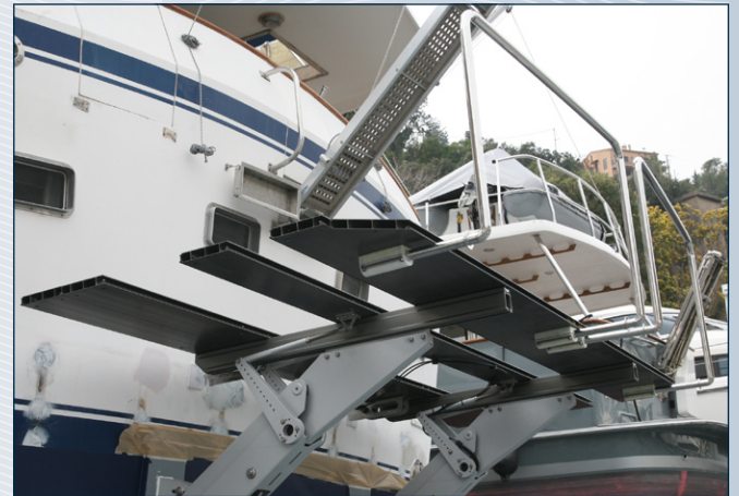
Displacement mechanics lifted position Platform lifted and retracted to the transom
