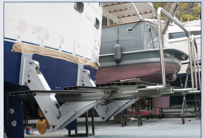
Displacement mechanics lowered position Platform fully extended at the bottom
